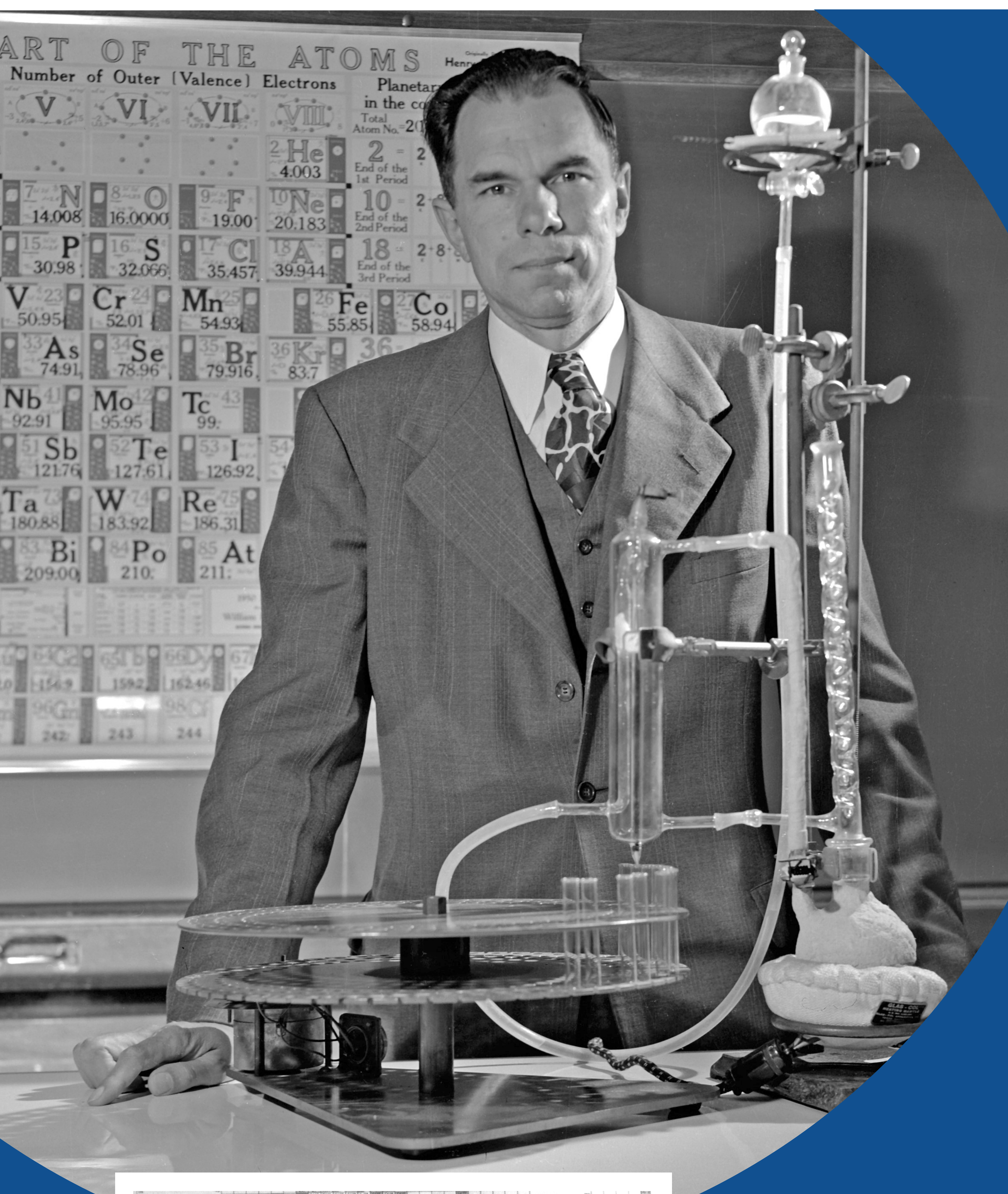
Glenn Seaborg using a Geiger-Muller counter. This counter supplies the high voltage to the GM tube and starts the count. The lead shield containing the detector and the sample is just above and to the right of his left hand.
