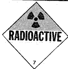
Figure D-1. Typical Radioactive Warning Placard
