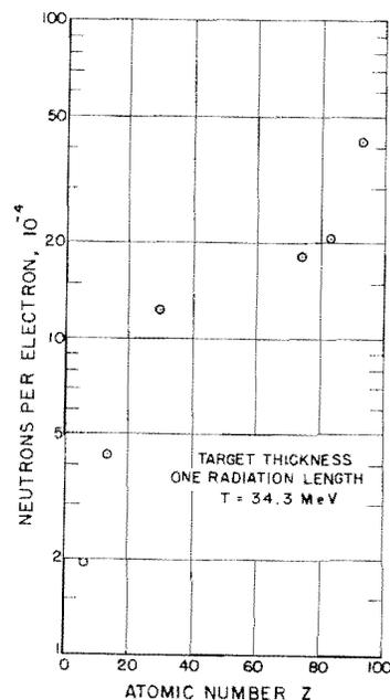
FIGURE 14. *Experimental yields of neutrons per incident 34.3 MeV electron for targets one radiation length thick as a function of atomic number Z.*
