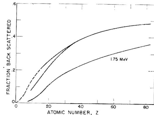
FIGURE 21. Fraction of incident back-scattered as a function of the atomic number  $Z$ .
