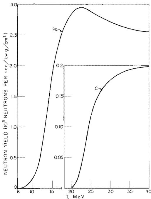
FIGURE 10. Relative neutron yield per kilowatt of bremsstrahlung from 1 gm/cm<sup>2</sup> targets of carbon and lead.
