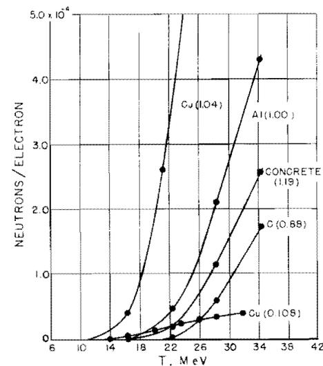
FIGURE 11. Yield of neutrons per incident electron as a function of initial electron energy for low- $Z$  elements.
