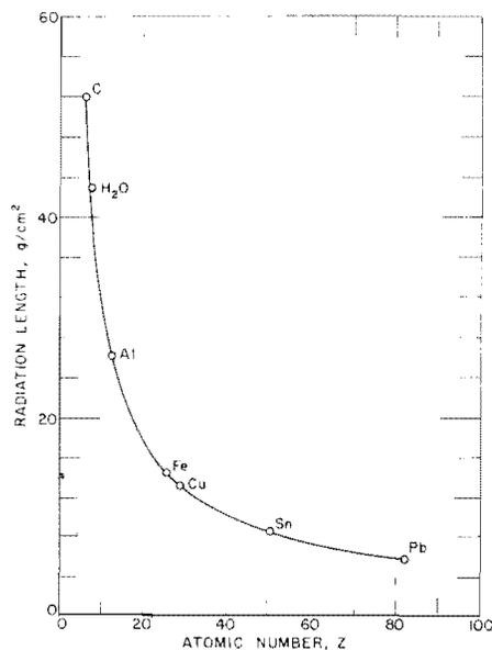
FIGURE 3. Radiation lengths in grams per square centimeter for various materials. Values given neglect effect of atomic electrons [6].
