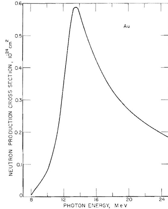
FIGURE 9. Neutron production cross section for gold. The curve represents  $\sigma_{in} = \sigma(\gamma, n) + 2\sigma(\gamma, 2n) + \sigma(\gamma, pn)$ . Data from ref. [14].
