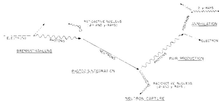
FIGURE 2. Interactions of radiation with matter.
