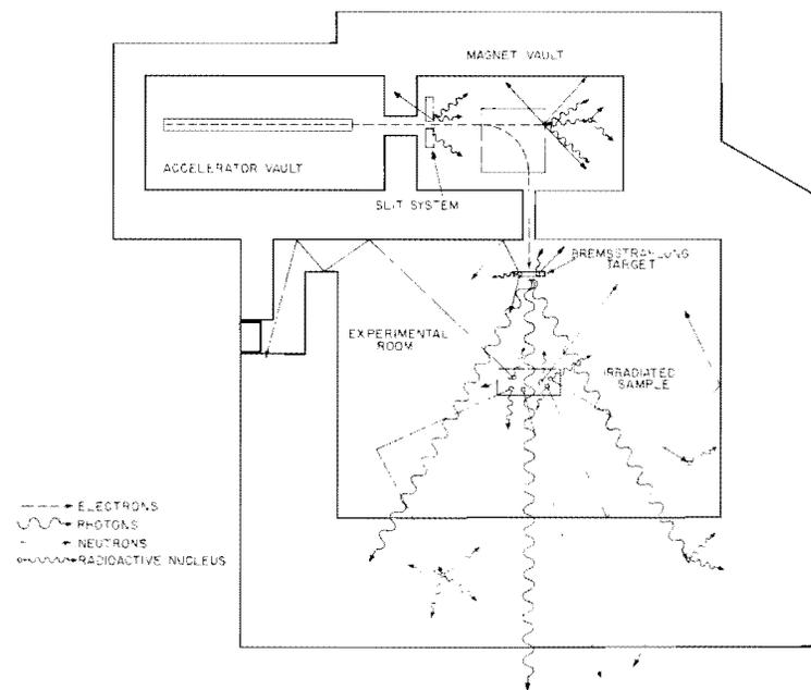
FIGURE 1. Schematic representation of an electron accelerator installation.
